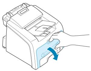
Pull the toner cartridge out and gently roll the cartridge 5 or 6 times to distribute the toner evenly inside the cartridge.
